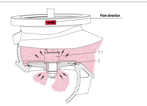
Valves with **balancing plugs** have to be installed with medium flowing over the plug (3) as indicated by flow direction arrow on valve body. <u>Working principles:</u>
